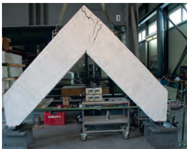
Fracture pattern of the test of a closing frame corner.
