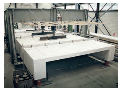
Fatigue test of bridge deck.
