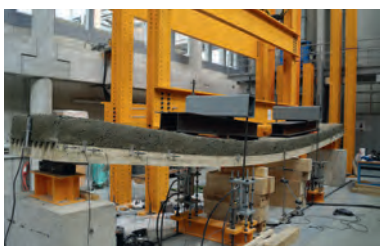
Timber-WCC slab in full-scale test.
