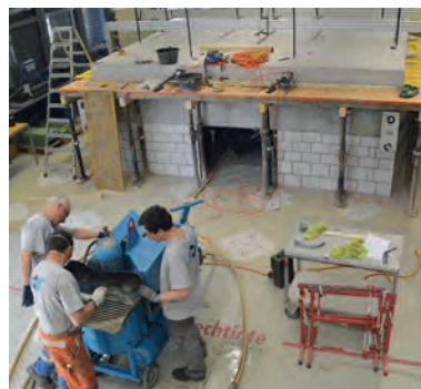
Pre-tensioned double-span slab: injection of tension cables.
