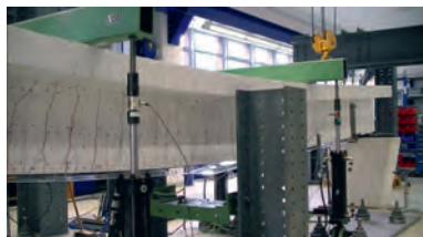
Four-point bend test of the untensioned beam strengthened with CRFP tensoning system.
