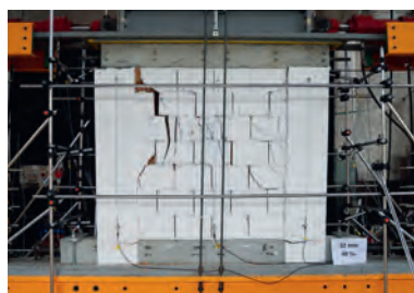
Cyclic test on masonry wall element with U-shaped corner strengthening made of thin UHPFRC layers.
